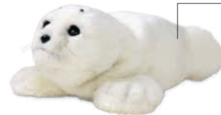
PARO A moving, feeling, 'healing pet'. Perfect as a companion for the disabled or elderly, Paro can sense the time of day, recognise its name and change facial expressions
